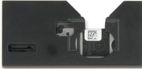
nanoDot slides in and out of the adapter (2D bar code facing front) for read-out in an original microStar reader
