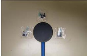
Field 1. ROOS chamber, TLDs and OSLDs on the solid water phantom for TBI dosimetry
