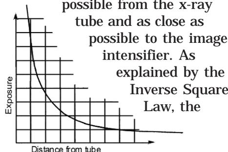
patient's exposure increases exponentially the closer he or she is placed to the x-ray tube. For example, assuming a source-to-image distance of 35 inches, an exposure rate of 7 R/minute at 23 inches from the x-ray source would increase to 26 R/minute at 12 inches from the source.
