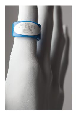
LANDAUER's ring dosimetry service provides comprehensive extremity radiation monitoring for workers required to manually manipulate or work in close proximity to radioactive materials and radiation producing equipment.
